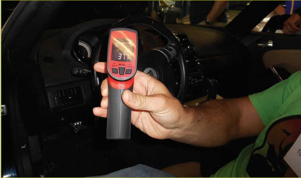
FIGURE 2—Air Duct Temperature (Courtesy of Dr. John Kershaw)
