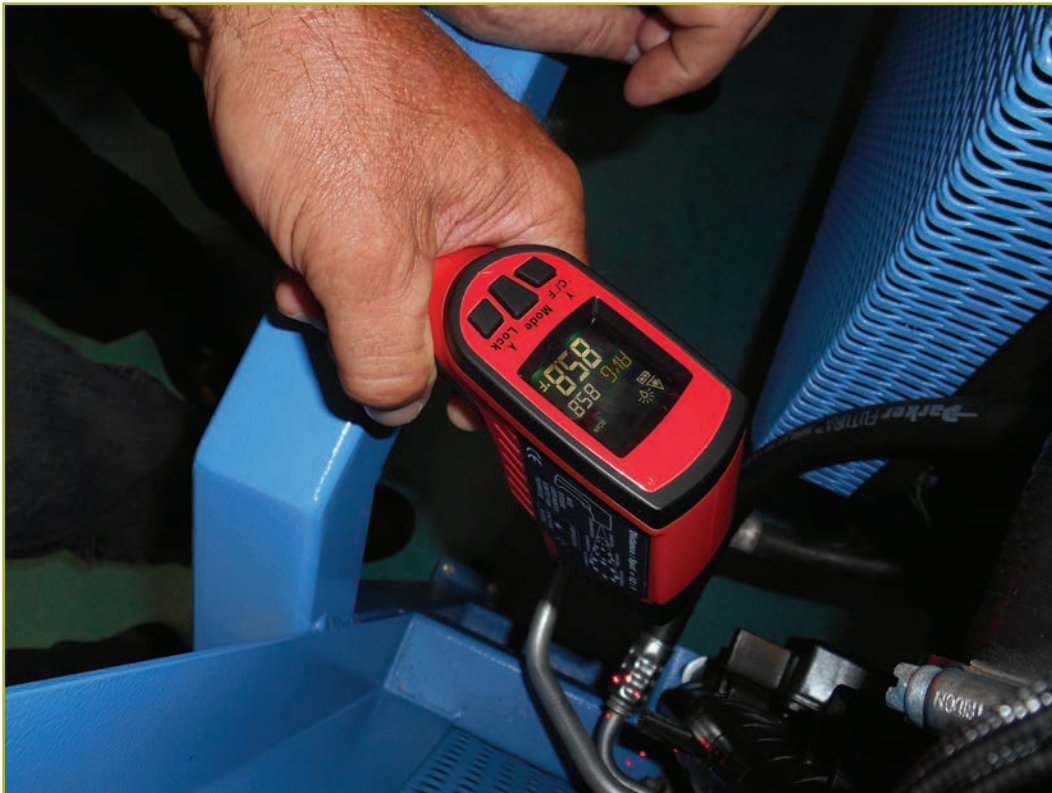
FIGURE 1—Measuring the Temperature of Refrigerant Entering the Condenser (Courtesy of Dr. John Kershaw)
